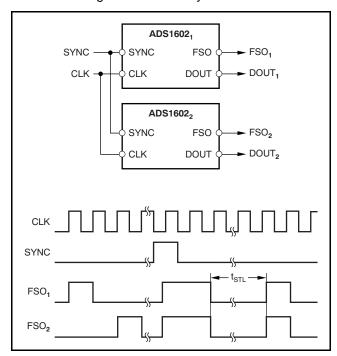
Figure 46. Synchronizing Multiple Converters
