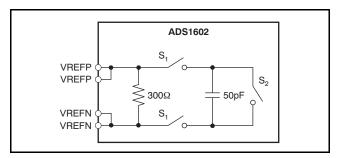
Figure 44. Conceptual Internal Circuitry for the Reference When REFEN = High
