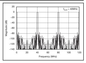
Figure 51. Frequency Response Out to 120MHz
