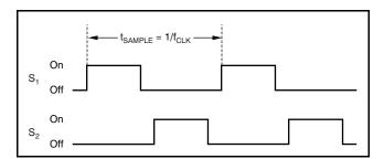
Figure 40. Timing for the Switches in Figure 39
