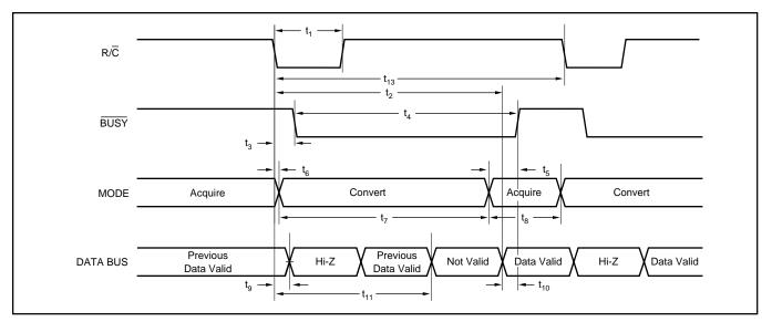
FIGURE 3. Conversion Timing with Outputs Enabled after Conversion ( $\overline{CS}$  Tied LOW.)
