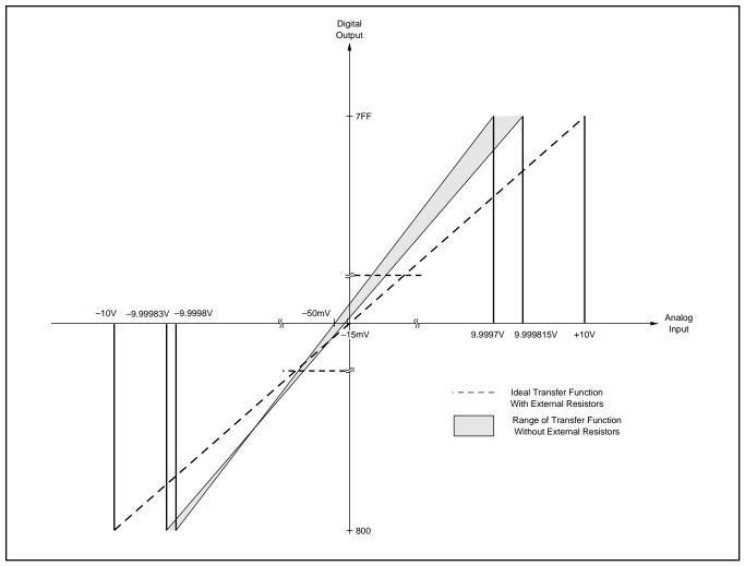
FIGURE 7. Full Scale Transfer Function.
