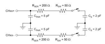
Figure 1. Equivalent Input Circuit
