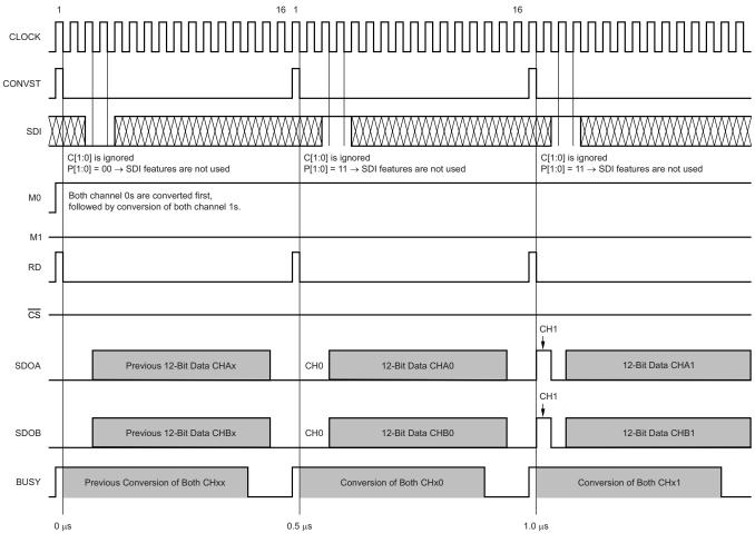
Figure 35. Mode III Timing Diagram (M0 = 1, M1 = 0)
