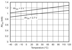
Figure 29. ANALOG SUPPLY CURRENT vs TEMPERATURE (Auto-NAP Mode)
