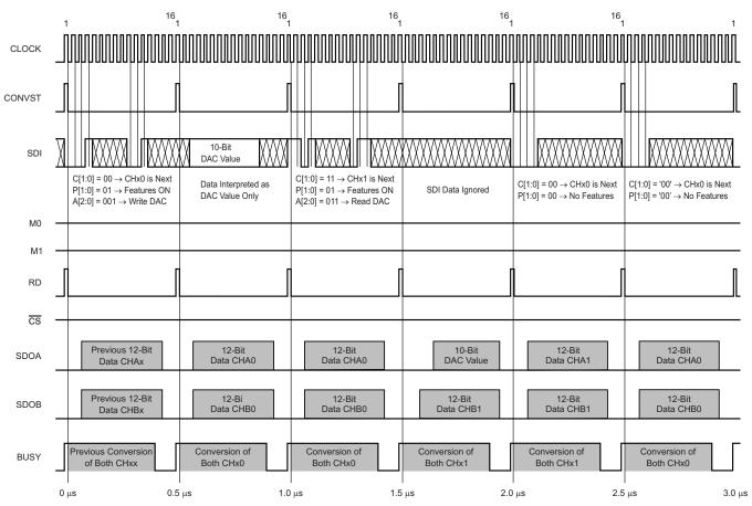
Figure 41. DAC Write and Read Access Timing Diagram
