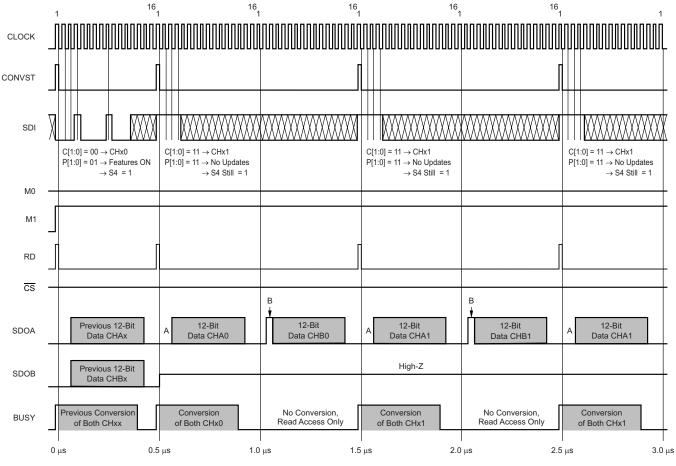
Figure 37. Special Mode II Timing Diagram (M0 = 0, M1 = 1, S4 = 1)
