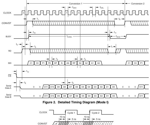
NOTE: All CONVST commands that occur more than 10 ns before the cycle 1 rising edge of the external clock (region A) initiate a conversion on the cycle 1 rising edge. All CONVST commands that occur 5 ns after the cycle 1 rising edge or 10 ns before the cycle 2 rising edge (region B) initiate a conversion on the cycle 2 rising edge. All CONVST commands that occur 5 ns after the cycle 2 rising edge (region C) initiate a conversion on the rising edge of the next clock period.
