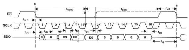
Figure 1. ADS7884 Interface Timing Diagram
