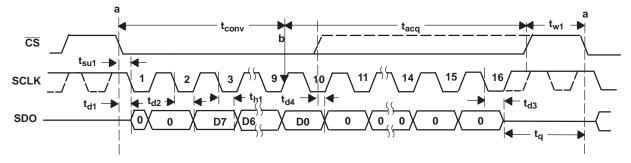
Figure 2. ADS7885 Interface Timing Diagram
