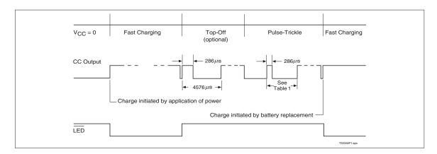
Figure 4. Charge Cycle Phases
