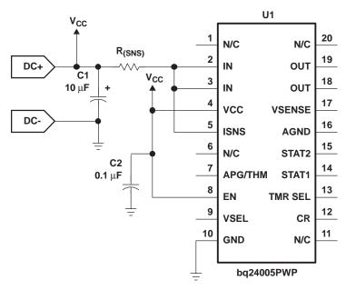
Figure 19. Current Sensing Circuit
