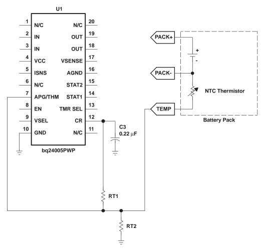
Figure 16. Temperature Sensing Circuit
