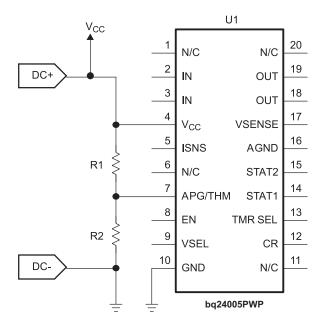
Figure 18. APG Sensing Circuit
