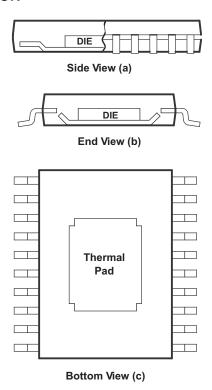
Figure 20. Views of Thermally Enhanced PWP Package
