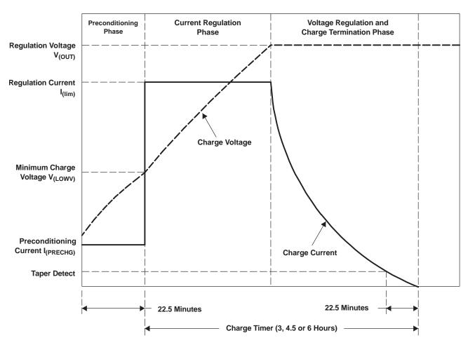
Figure 14. Typical Charge Profile
