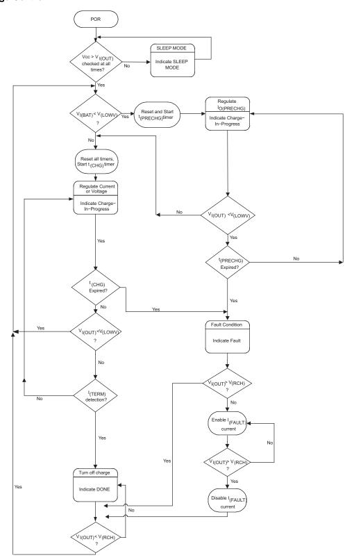
Figure 6. Charge Control Operational Flow Chart
