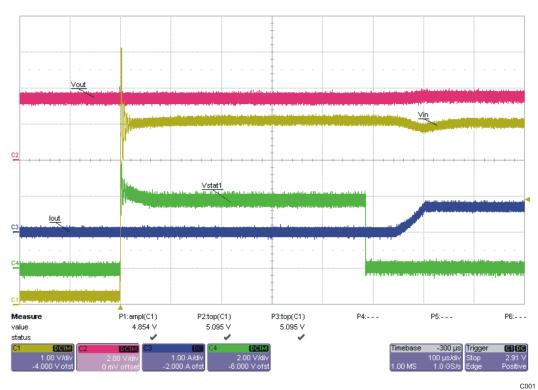
Figure 2. V<sub>IN</sub> Hot-Plug Power-Up Sequence
