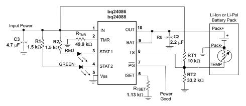
Figure 18. bq24086 and bq24088 Application Schematic
