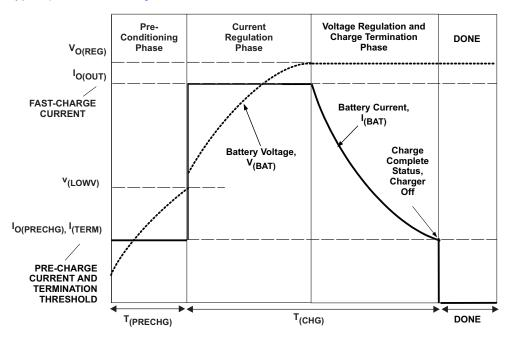
Figure 8. Charging Profile With T<sub>J(REG)</sub>
