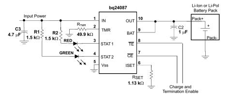
Figure 22. bq24087 Application Schematic
