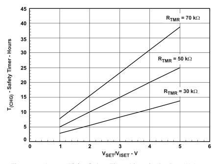
Figure 13. bq24085/6/78 Safety Timer Linearity for R<sub>TMR</sub> Values
