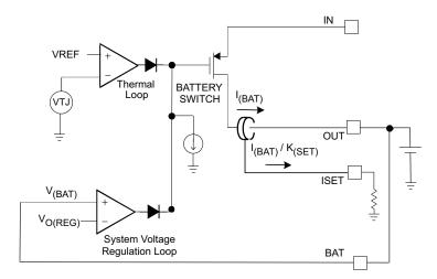
Figure 9. Thermal Regulation Circuit
