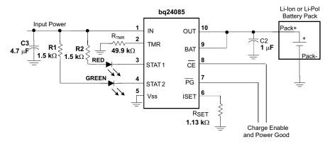
Figure 21. bq24085 Application Schematic
