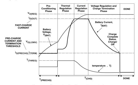
Figure 10. Charge Profile, Thermal Loop Active
