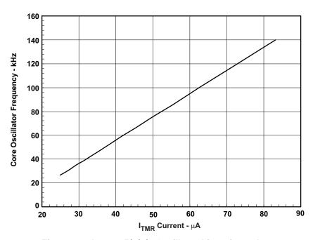
Figure 14. bq24085/6/7/8 Oscillator Linearity vs  $I_{TMR}$   $R_{TMR}$  30  $K\Omega$  - 100  $K\Omega$
