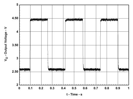
Figure 15. Battery-Absent Detection Waveforms
