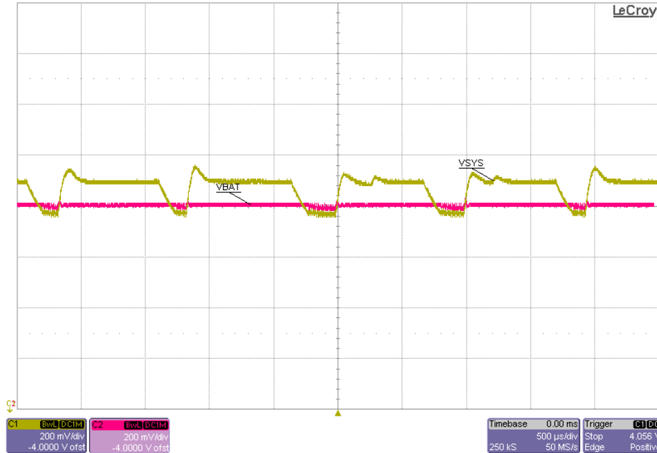
Figure 8-7. V(SYS) When Reverse Boost Prevention Circuit is Active
