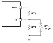
Figure 9-5. TS Resistor Network
