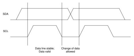
Figure 9-12. Bit Transfer on the I<sup>2</sup>C Bus
