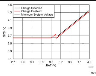
Figure 9-7. System Voltage vs Battery Voltage
