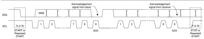
Figure 9-14. Data Transfer on the I<sup>2</sup>C Bus
