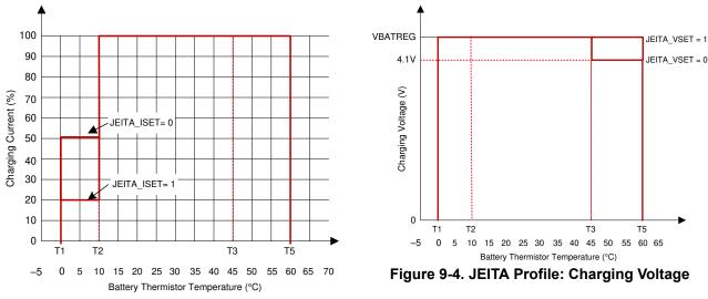
Figure 9-3. JEITA Profile: Charging Current
