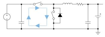
Figure 10-1. High Frequency Current Path
