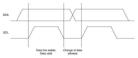
Figure 9-8. Bit Transfer on the I<sup>2</sup>C Bus
