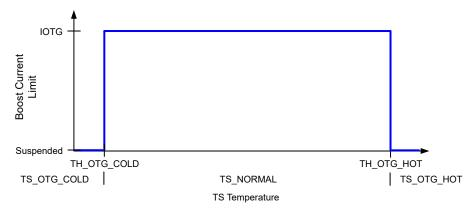
Figure 9-5. TS Pin Thermistor Sense Threshold in Boost Mode
