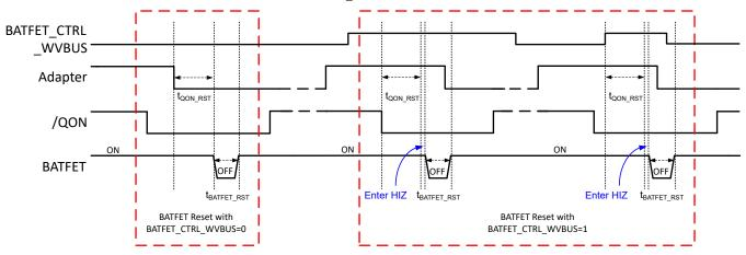
Figure 9-6. System Power Reset Timing
