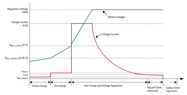
Figure 9-2. Battery Charging Profile
