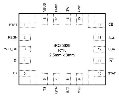
Figure 7-2. BQ25629 Pinout, 18-Pin WQFN Top View
