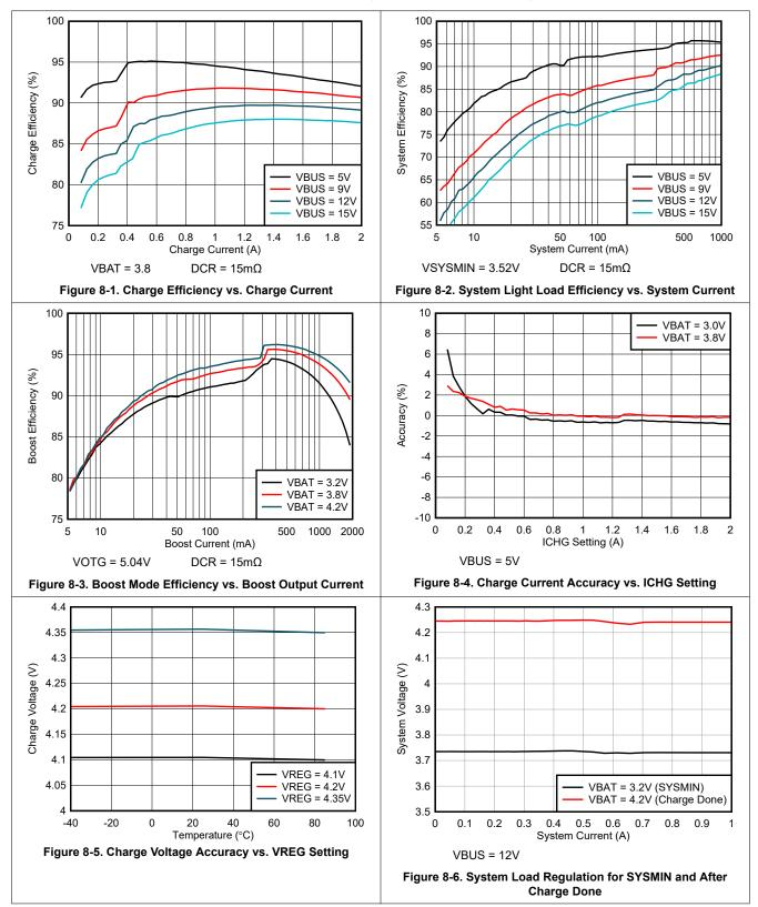
C<sub>VBUS</sub> = 1µF, C<sub>PMID</sub>= 10µF, C<sub>SYS</sub>= 20µF, C<sub>BAT</sub>= 1µF, L= 1µH (unless otherwise specified)
