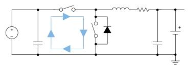
Figure 12-1. High Frequency Current Path
