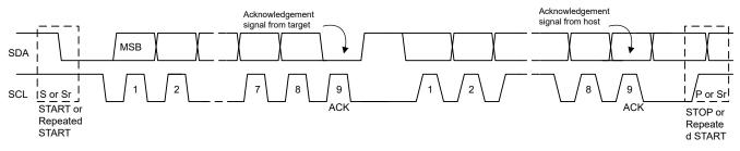
Figure 9-10. Data Transfer on the I<sup>2</sup>C Bus
