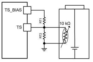
Figure 9-4. TS Resistor Network
