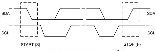
Figure 9-9. START and STOP Conditions on the I<sup>2</sup>C Bus
