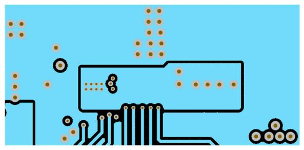
Figure 12-3. Layout Example: Inner Layer 3 (AGND pour; SW node pour; signal routing)
