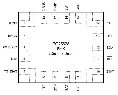
Figure 7-1. BQ25628 Pinout, 18-Pin WQFN Top View
