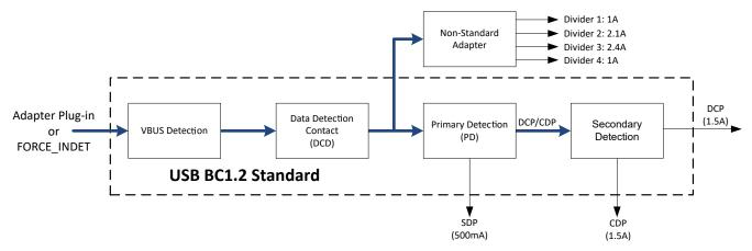
Figure 9-1. D+/D– Detection Flow
