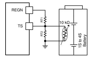
Figure 8-12. TS Resistor Network
