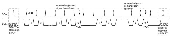
Figure 8-17. Data Transfer on the I<sup>2</sup>C Bus
