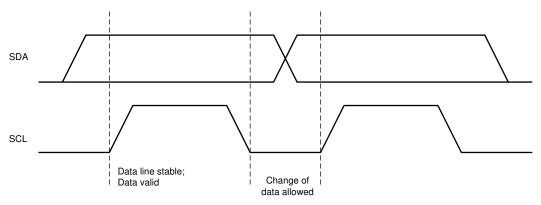
Figure 8-15. Bit Transfers on the I<sup>2</sup>C Bus
