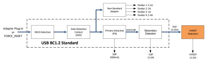
Figure 8-1. D+/D– Detection Flow
