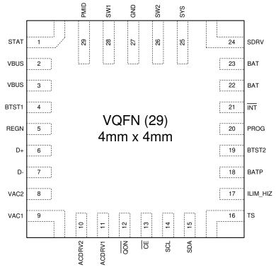
Figure 6-1. RQM Package 29-Pin VQFN Top View
