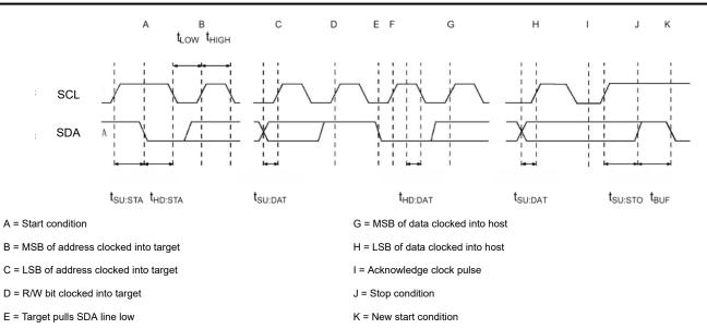
Figure 9-7. I<sup>2</sup>C Read Timing
