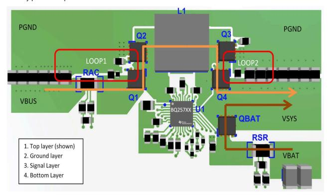
Figure 12-1. Buck-Boost Charger Layout Reference Example Top View
