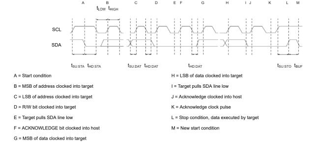
Figure 9-6. I<sup>2</sup>C Write Timing
