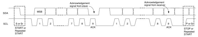
Figure 9-10. Data Transfer on the I<sup>2</sup>C Bus
