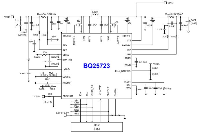
Figure 10-1. Application Diagram of BQ25723
