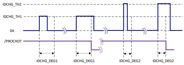
Figure 9-1. Two-Level Battery Discharging Current Trigger PROCHOT Diagram
