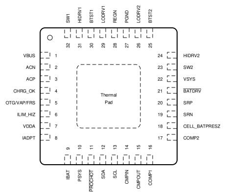
Figure 7-1. RSN Package 32-Pin WQFN Top View
