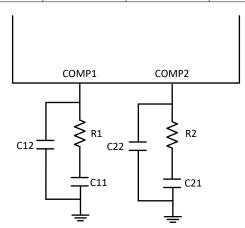
Figure 9-2. Compensation RC Network
