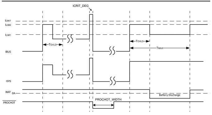
Figure 9-3. Two-Level Adapter Current Limit Timing Diagram
