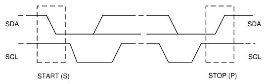
Figure 30. START and STOP Conditions on the I<sup>2</sup>C Bus
