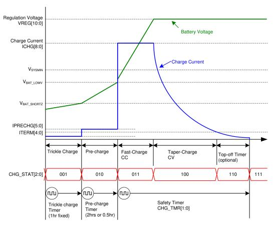
Figure 23. Battery Charging Profile
