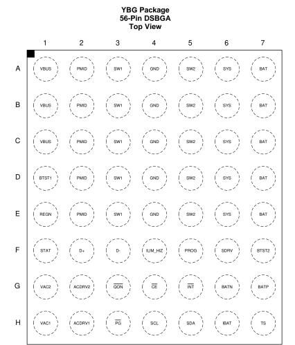
Top View = Xray through a soldered down part with A1 starting in upper left corner
