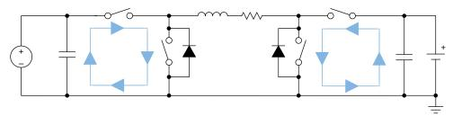
Figure 112. Buck-Boost Converter High Frequency Current Path
