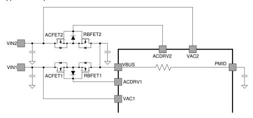
Figure 15. Two ACFETs-RBFETs Structure Supporting One Input at VAC1 and One Input at VAC2
