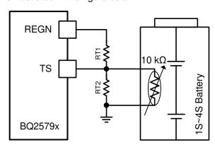
Figure 25. TS Resistor Network
