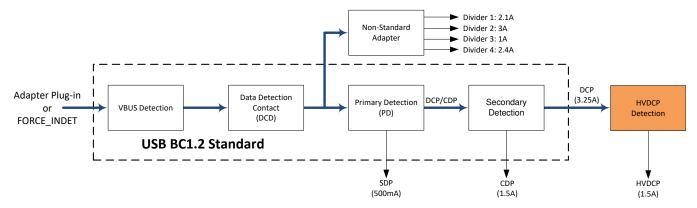
Figure 18. D+/D- Detection Flow
