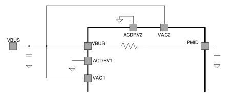
Figure 13. Single Input Connected to VBUS Directly Without ACFET-RBFET
