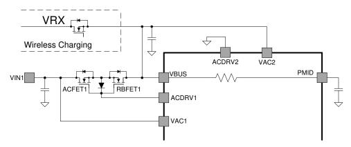
Figure 14. One ACFET-RBFET Structure Supporting One Input at VAC1 and/or One Input at VBUS
