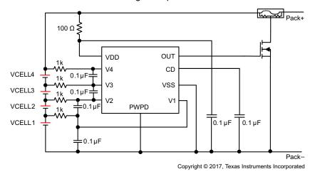
Figure 9-1. Application Configuration for Active High
