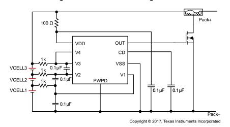
Figure 9-3. 3-Series Cell Configuration
