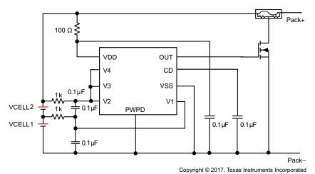
Figure 9-2. 2-Series Cell Configuration
