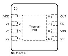
Figure 6-1. DSG Package 8-Pin WSON Top View
