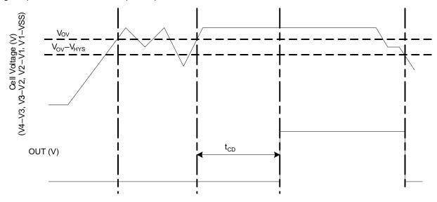
Figure 8-1. Timing for Overvoltage Sensing (OUT Pin Is Active High)
