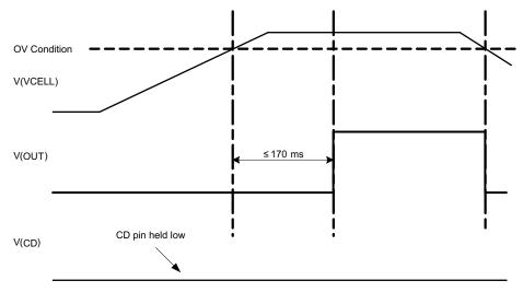
Figure 8-3. Timing for Customer Test Mode
