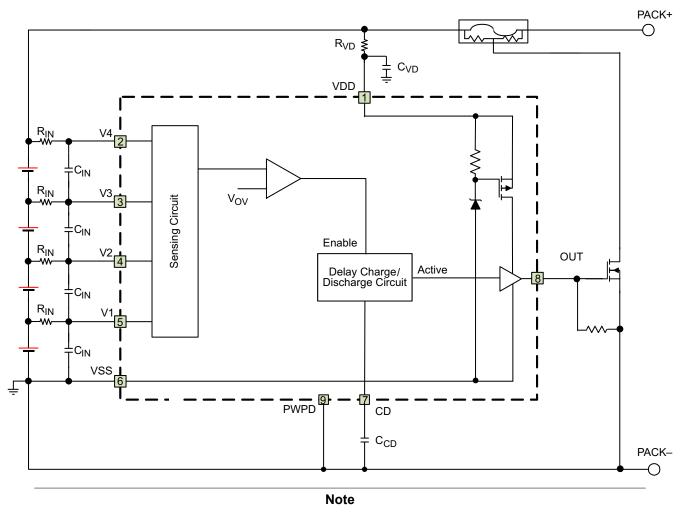
In the case of an Open Drain Active Low configuration, an external pull-up resistor is required on the OUT terminal.
