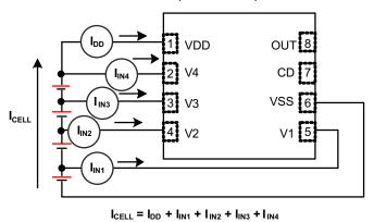
Figure 8-4. Configuration for IC Current Consumption Test
