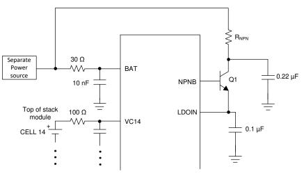
Figure 10-4. Separate Power Source to BAT
