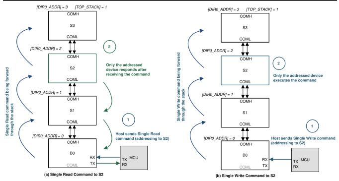
Figure 9-28. Single Device Read/Write
