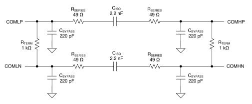
Components Required for Cap Coupled Daisy Chain on the same PCB
