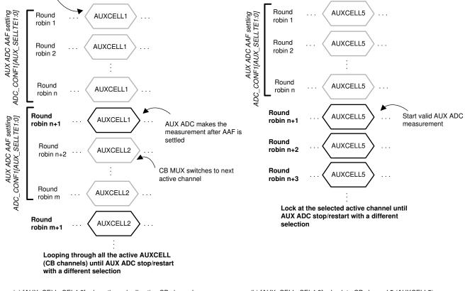
(a)  $[AUX\_CELL\_SEL4:0] = loop through all active CB channels$
