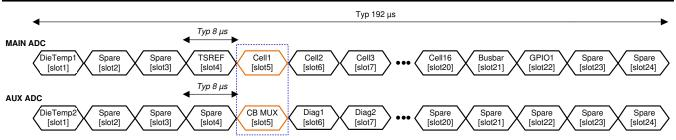
a) [AUX\_CELL\_SEL] = 00h – Running all active cell channels set by ACTIVE\_CELL\_CONF register. Ch1 conversion.
