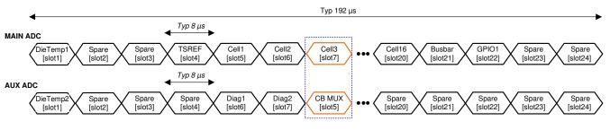
c) [AUX\_CELL\_SEL] = 04h – Lock to AUX CELL 3. Ch3 conversion.
