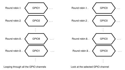
(a) [AUX\_GPIO\_SEL3:0] = loop through all GPIO channels
