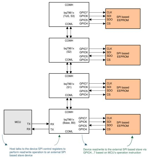
Figure 9-39. SPI Master Stack Configuration
