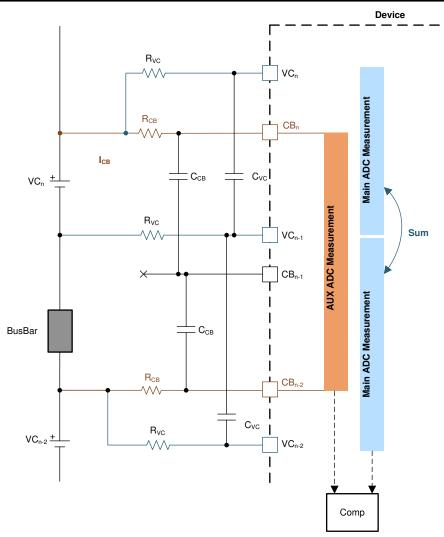
Figure 9-58. Cell Measurement Check with Bus Bar Connected to Individual VC Channel
