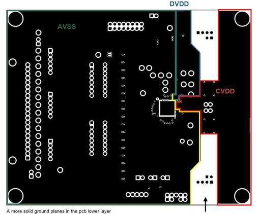
Daisy chain circuit components: Keepout area with no other traces or ground plans
