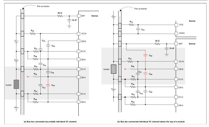
Figure 9-56. Bus Bar Connected to Individual VC Channel
