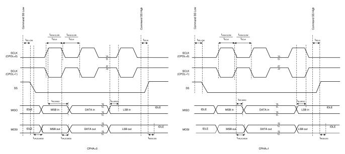
Figure 9-41. SPI Master Timing Diagram
