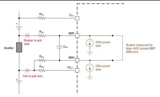
Figure 9-55. Current Sink for BBP/N Open Wire Detection
