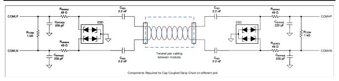
Figure 10-7. Capacitor Isolation on Different PCB
