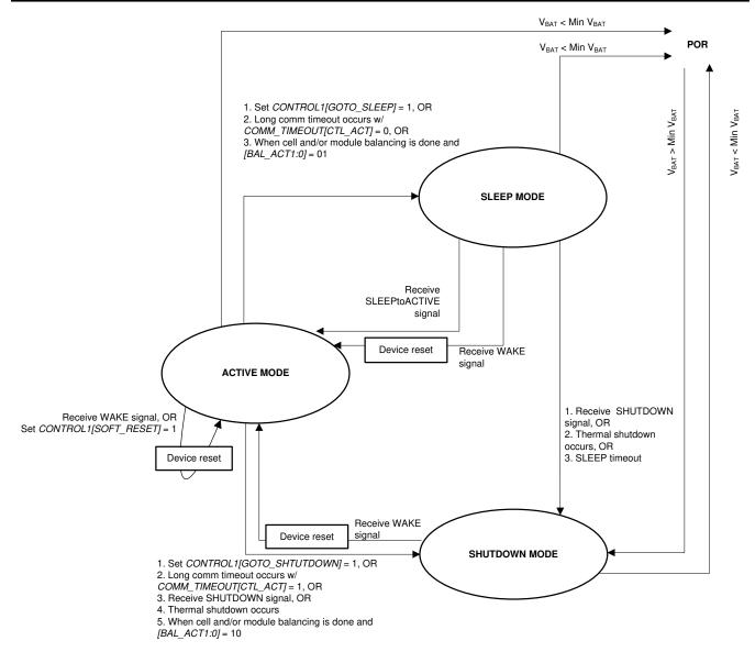
Figure 9-59. Power State Diagram
