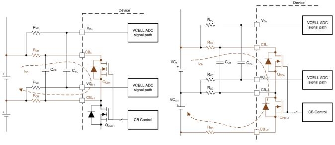
(a) Cell balancing with internal CBFET
