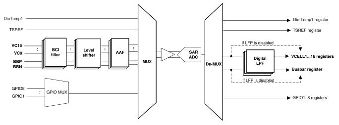
Figure 9-2. Main ADC Measurement Path
