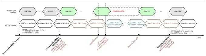
Figure 9-17. Cell Balancing Pause and Resume by OTCB Detection
