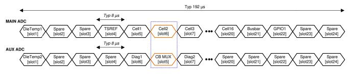
b) [AUX\_CELL\_SEL] = 00h - Running all active cell channels set by ACTIVE\_CELL\_CONF register. Ch2 conversion.
