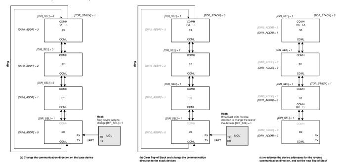
Figure 9-37. Example to Change Communication Direction in Daisy Chain
