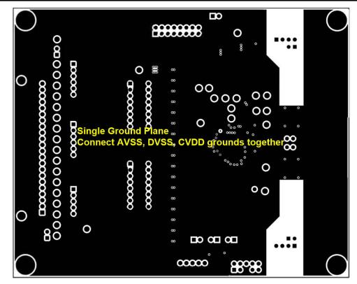
Figure 12-6. ThIrd Layer with Single Ground Plane
