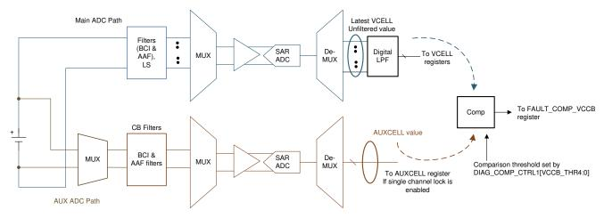
Figure 9-47. Cell Voltage Measurement Diagnostic
