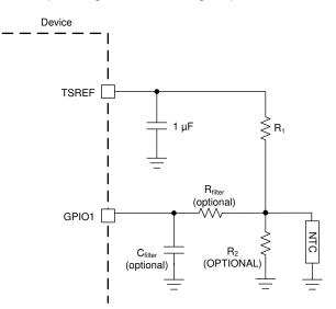
Figure 9-6. Thermistor Connection
