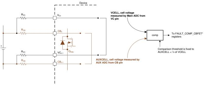
Figure 9-50. Cell Balancing FET Diagnostic
