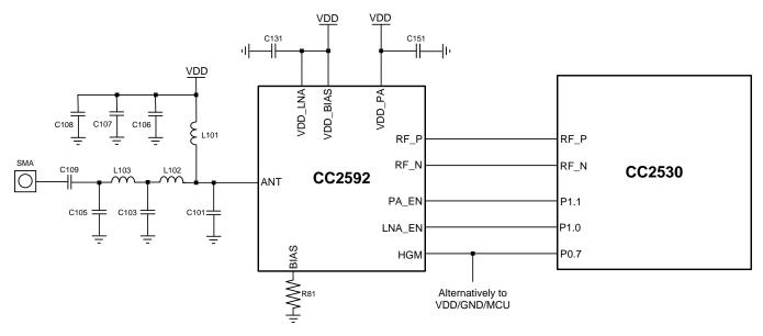
Figure 9-1. Application Circuit Example for CC2530 + CC2592
