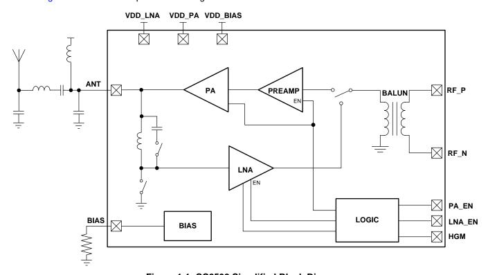
Figure 1-1. CC2592 Simplified Block Diagram
