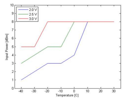
Figure 7-1. Maximum Recommended Drive Level
