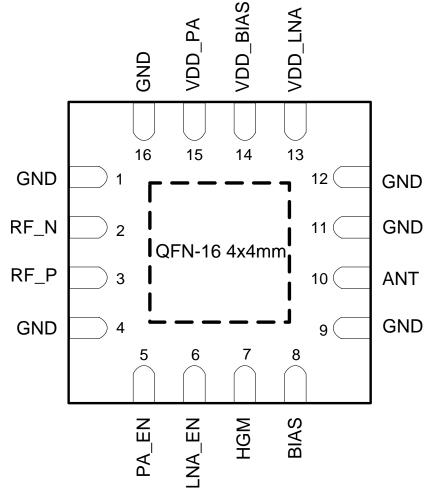
Figure 3-1. Terminal Top View
