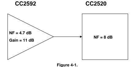
The noise factor of a system consisting of the CC2592 device and a CC2520 device, as seen in Figure 4-1 is given by:
