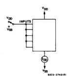
Fig. 11-Quiescent-device-current test circuit.
