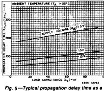
Fig. 5—Typical propagation delay time as a function of load capacitance, (CLOCK to Q).
