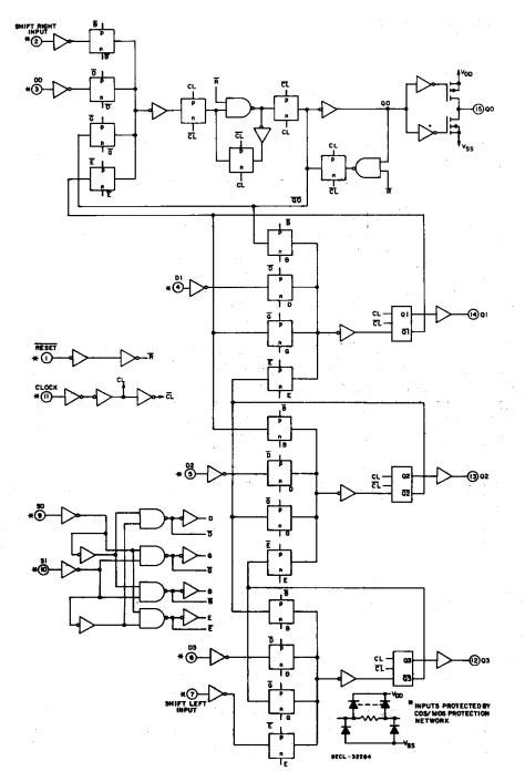
Fig. 8—CD40194B logic diagram.
