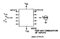
Fig. 10 - Input voltage test circuit.
