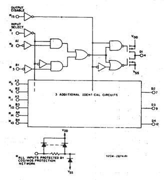
Fig. 1 - Logic diagram for CD40257B.
