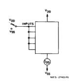
Fig.11 - Quiescent device current test circuit.
