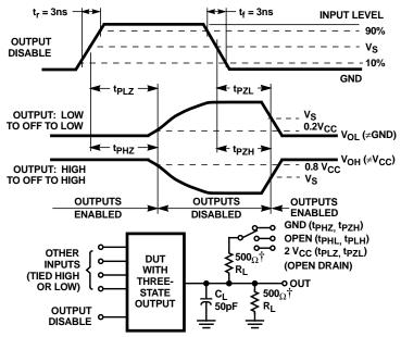
†FOR AC SERIES ONLY: WHEN V<sub>CC</sub> = 1.5V, R<sub>L</sub> = 1k $\Omega$
