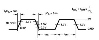
NOTE: Outputs should be switching from 10% V<sub>CC</sub> to 90% V<sub>CC</sub> in accordance with device truth table. For  $f_{MAX}$ , input duty cycle = 50%.
