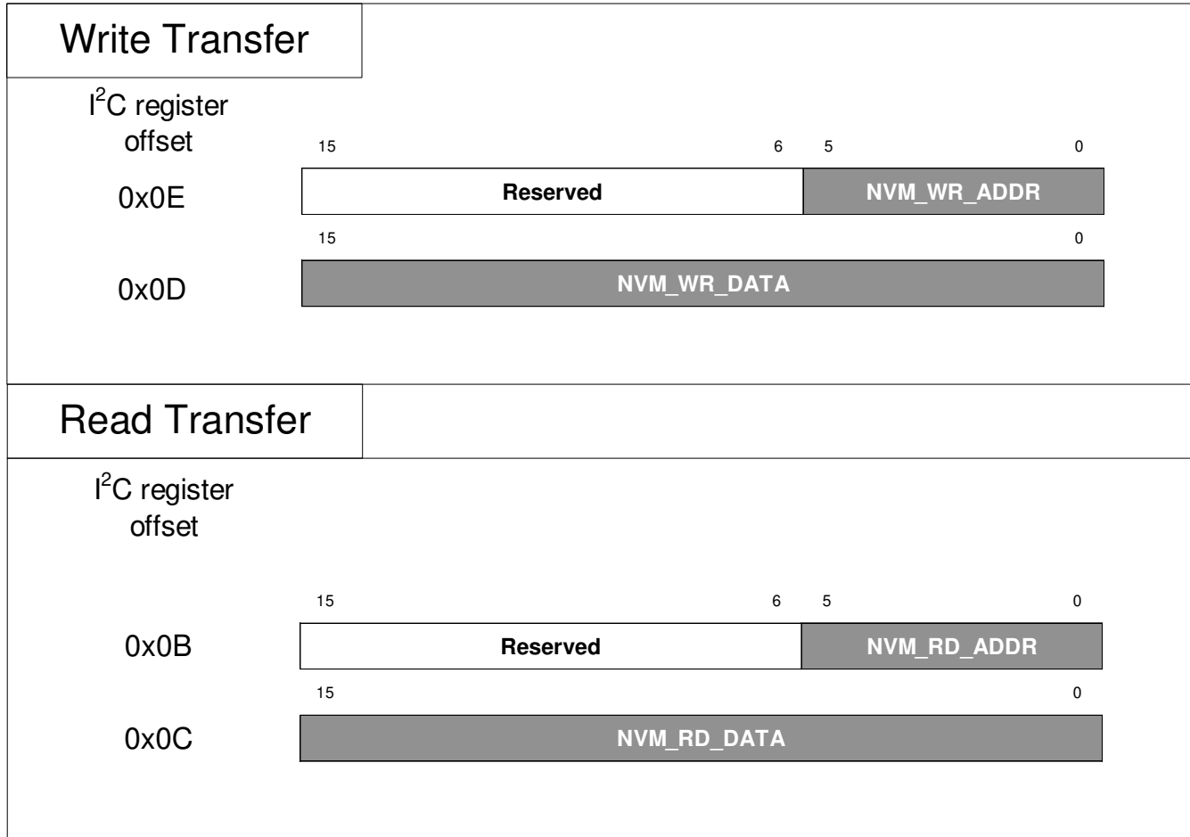
Figure 9-12. EEPROM Direct Access Using I 2 C
