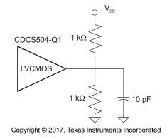
Figure 4. Test Load
