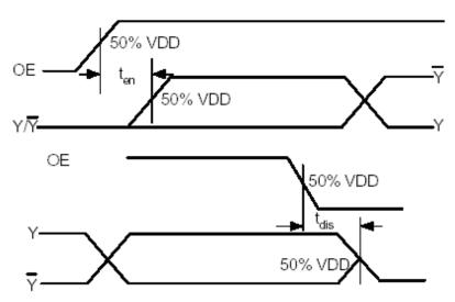
Figure 11. Time Delay Between OE and Clock Output  $(Y, \overline{Y})$
