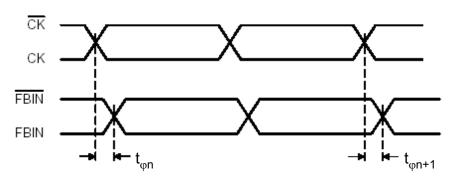
Figure 5. Static Phase Offset
