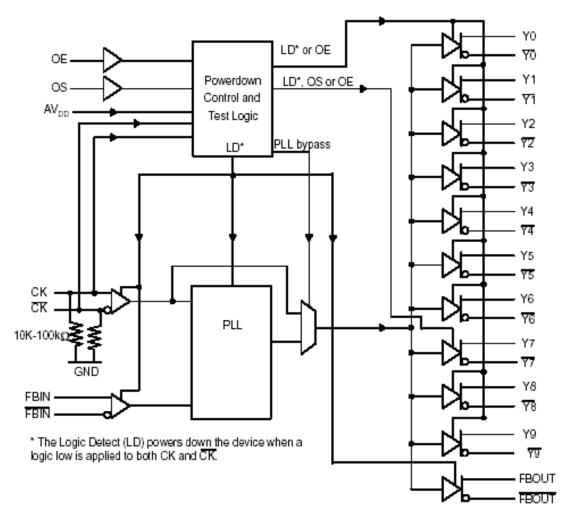
Figure 1. LOGIC DIAGRAM (POSITIVE LOGIC)
