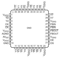
40-pin HP-VFQFP-N (6,0 x 6,0 mm Body Size, 0,5 mm Pitch, M0#220, Variation VJJD-2, E2 = D2 = 2,9 mm  $\pm$  0,15 mm) Package Pinouts
