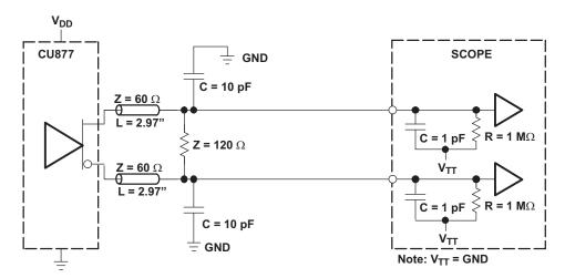
Figure 2. Output Load Test Circuit 1
