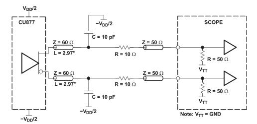
Figure 3. Output Load Test Circuit 2
