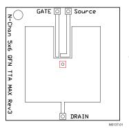
Max  $R_{\theta JA} = 50^{\circ}\text{C/W}$  when mounted on 1 in<sup>2</sup> (6.45 cm<sup>2</sup>) of 2-oz (0.071-mm) thick Cu.
