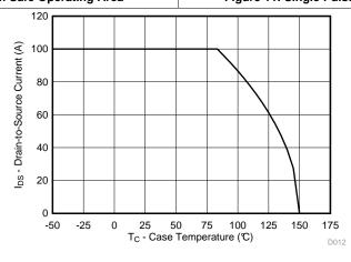
Figure 12. Maximum Drain Current vs Temperature
