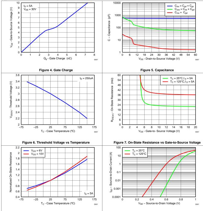
Figure 8. Normalized On-State Resistance vs Temperature
