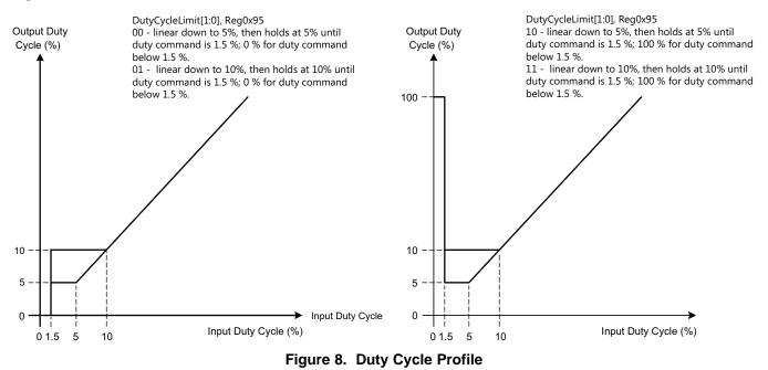
The speed command may not always be equal to the PWM\_DCO because the DRV10987 device has the AVS function (see *Anti-Voltage Surge Function*), the software current-limit function (see *Software Current Limit*), and the closed-loop accelerate function (see *Closed-Loop Accelerate*) to optimize the control performance. These functions can limit the PWM\_DCO, which affects the output amplitude (see Figure 9).
