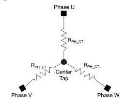
Figure 13. Wye-Connected Motor Phase Resistance
