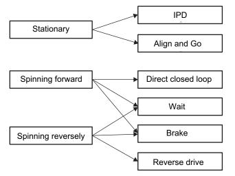
Figure 16. Start the Motor Under Different Initial Conditions
