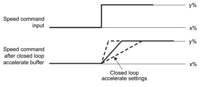
Figure 30. Closed-Loop Accelerate
