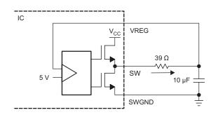
Step-Down Regulator With External Resistor (Linear Mode)
