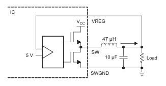
Step-Down Regulator With External Inductor (Buck Mode)
