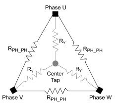
Figure 14. Delta-Connected Motor and the Equivalent Wye Connections
