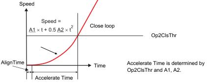
Figure 24. Motor Start-Up Process
