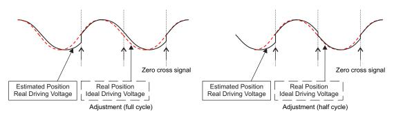
Figure 27. Closed-Loop Control Commutation-Adjustment Mode
