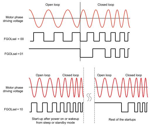
Figure 43. FG Behavior During Open Loop
