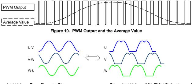
Sinusoidal Voltage From Phase to Phase
