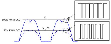
Figure 12. Output Voltage Amplitude Adjustment
