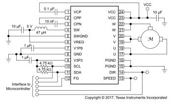
Figure 70. Typical Application Schematic
