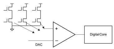
Figure 34. Lock-Detection Current Limit
