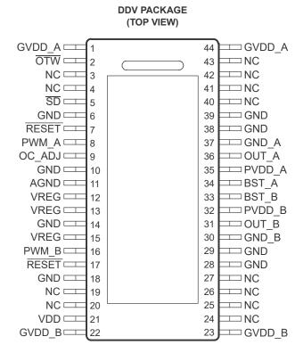
Figure 5-1. DDV Package 44-Pin HTSSOP PowerPad Top View
