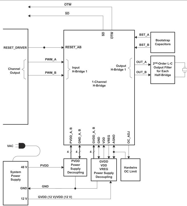
Figure 7-2. Functional Block Diagram
