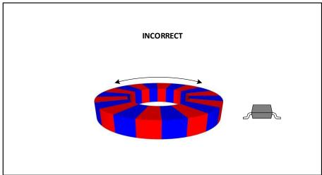
Figure 22. Correct and Incorrect Magnet Orientations
