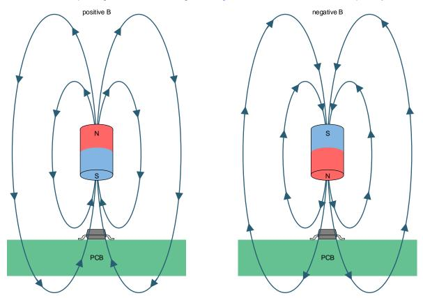
Figure 12. Flux Direction Polarity
