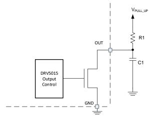
Figure 14. Open-Drain Output (Simplified)
