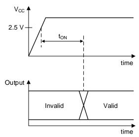
Figure 15. t<sub>ON</sub> Definition
