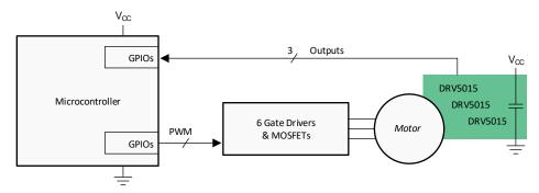
Figure 18. BLDC Motor System
