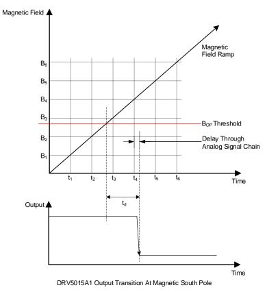
Figure 17. Propagation Delay
