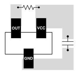
Figure 25. DRV5021-Q1 Layout Example
