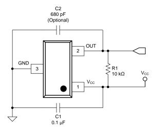
Figure 20. Proximity Sensing Circuit
