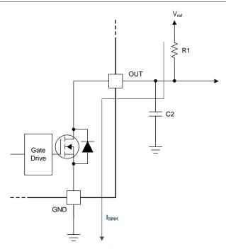
Figure 19. Open-Drain Output
