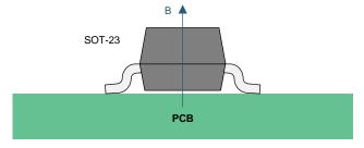
Figure 10. Direction of Sensitivity
