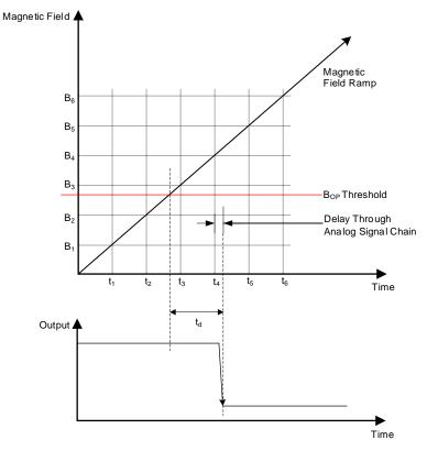
Figure 18. Propagation Delay
