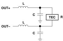
Figure 13. LC Output Filter
