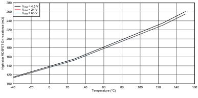
Figure 6-6. High-side FET on resistance
