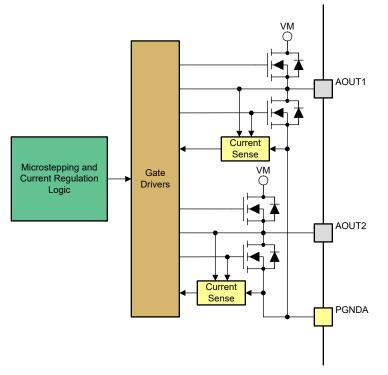
Figure 7-4. PWM Motor Driver Block Diagram
