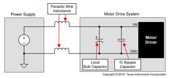
Figure 10-1. Example Setup of Motor Drive System With External Power Supply
