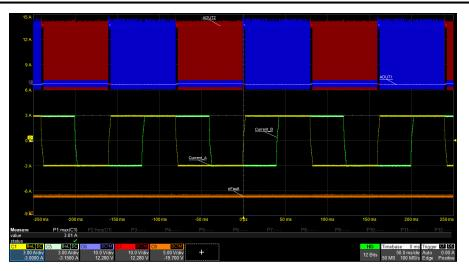
Figure 8-3. Full-step at 25 pps with  $\rm I_{FS}$  = 3 A
