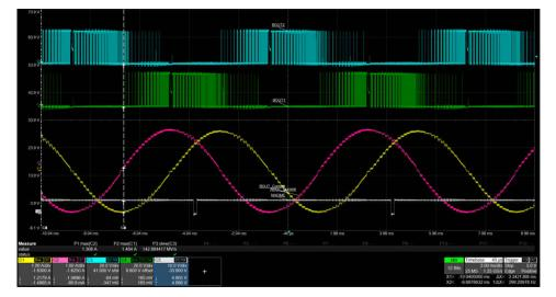
Traces from top to bottom: BOUT2, BOUT1, coil B current, coil A current, nHOME
