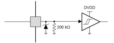
Figure 7-34. Logic-Level Input Pin Diagram
