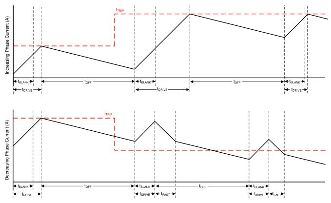
Figure 7-14. Smart tune Dynamic Decay Mode
