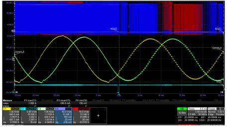
Traces from top to bottom: AOUT2, AOUT1, coil A current, coil B current, nSCS
