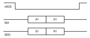
Figure 7-48. SPI Format - Standard "16-bit" Frame
