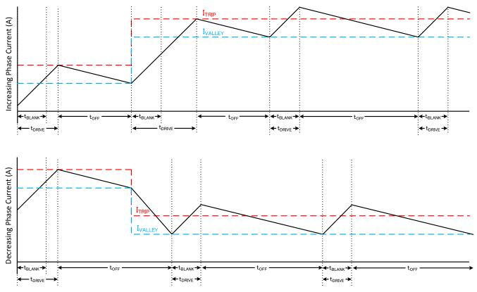
Figure 7-15. Smart tune Ripple Control Decay Mode
