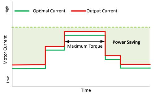
Figure 7-22. Power Saving with Auto-torque
