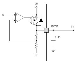
Figure 7-31. Linear Voltage Regulator Block Diagram
