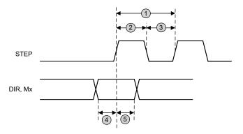
Figure 6-2. STEP and DIR Timing Diagram
