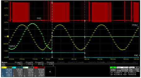
Figure 7-45. Coil B open-load detection
