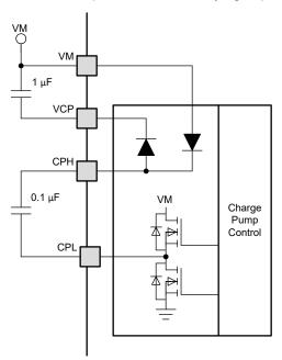
Figure 7-30. Charge Pump Block Diagram
