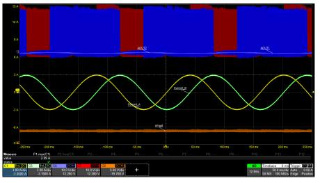
Figure 8-5. 1/256 microstepping at 6400 pps with  $I_{\text{FS}}$  = 3 A
