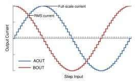
Figure 7-3. Full-Scale and RMS Current
