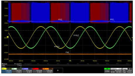
Figure 8-2. 1/16 microstepping at 400 pps with I<sub>FS</sub> = 3 A
