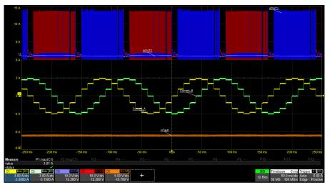
Figure 8-4. 1/4 microstepping at 100 pps with  $I_{\text{FS}}$  = 3 A
