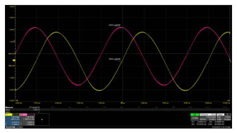
Figure 7-19. Coil Current Waveform with Silent Step Decay
