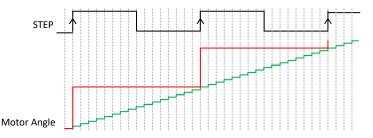
Figure 7-7. Automatic Microstepping Interpolation
