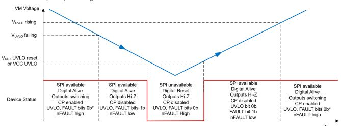
\* FAULT bit will be 0b if no fault is present
