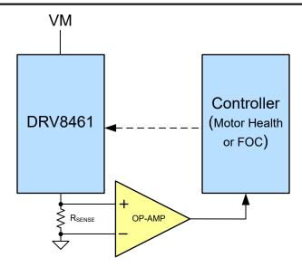
Figure 7-16. Current Sensing with External Resistor
