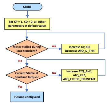
Figure 7-28 is the flowchart for selecting PD control loop parameters.
