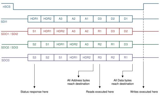
Figure 7-50. SPI Frame With Three Devices
