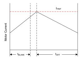
Figure 7-10. Current Chopping Waveform
