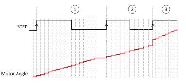
Figure 7-8. Automatic Microstepping with Changing STEP Frequency
