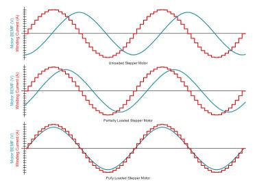
Figure 7-42. Stall Detection by Monitoring Motor Back-EMF
