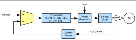
Figure 7-17. Silent step block diagram
