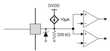
Figure 7-32. Tri-Level Input Pin Diagram
