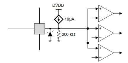
Figure 7-33. Quad-Level Input Pin Diagram
