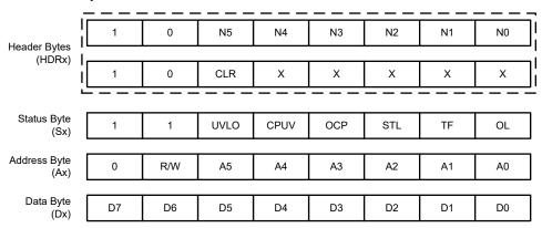
Figure 7-53. Contents of Header, Status, Address, and Data Bytes
