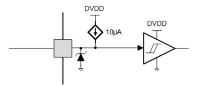
Figure 7-35. nSCS Input Pin Diagram
