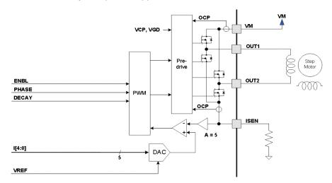
Figure 3. Motor Control Circuitry
