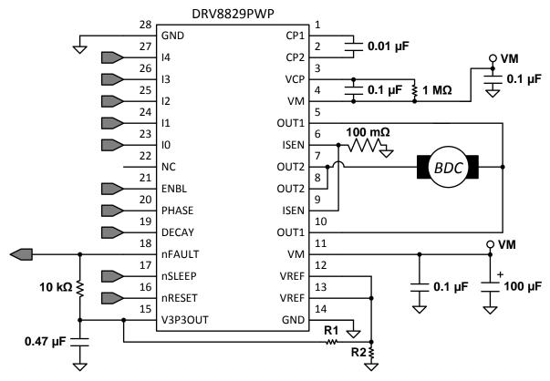
Figure 5. Typical Application Schematic
