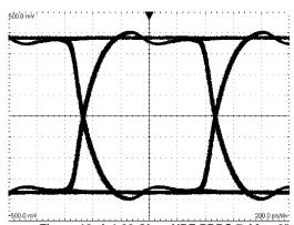
Figure 12. A 1.06 Gbps NRZ PRBS-7 After 2" Differential FR-4 Stripline V:100 mV / DIV, H:200 ps / DIV
