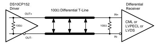
Figure 9. Typical DS10CP152Q Output DC-Coupled Interface to an LVDS, CML or LVPECL Receiver
