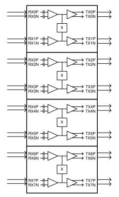
Figure 8-1. Block diagram showing all four 2x2 cross-points in the DS280MB810
