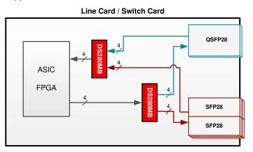
Figure 9-5. Front-port application block diagram
