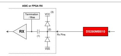
Figure 9-2. Considerations for DC coupling to ASIC RX
