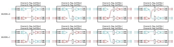
Figure 8-3. Signal distribution configuration options when using pin-control mode (channel A can be 0, 2, 4, or 6; channel B can be 1, 3, 5, or 7)
