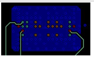
Figure 11-6. Microstrip Example, Internal Signal Layer 1
