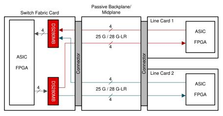
Figure 9-3. Typical backplane and mid-plane application block diagram
