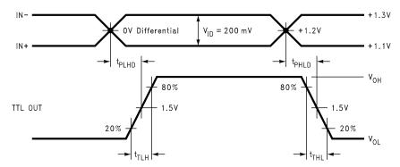
Figure 4. Receiver Propagation Delay and Transition Time Waveforms
