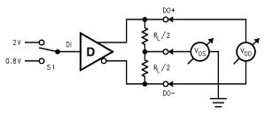
Figure 2. Differential Driver DC Test Circuit
