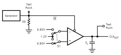
Figure 3. Output Enable (OE) Delay Test Circuit
