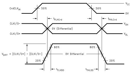
Figure 7. Driver Propagation Delay and Transition Time Waveforms
