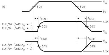
Figure 11. Driver TRI-STATE Waveforms
