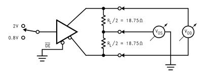
Figure 5. Differential Driver DC Test
