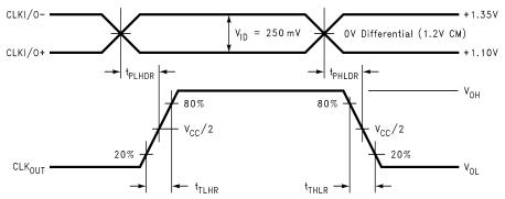
Generator waveform for all test unless otherwise specified: f = 25 MHz, 50% Duty Cycle, Zo =  $50\Omega$ , t<sub>TLH</sub> = 1 ns, t<sub>THL</sub> = 1 ns.
