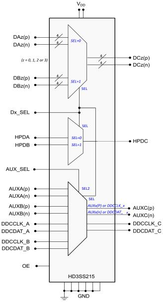
The high speed data ports incorporate  $20k\Omega$  pull down resistors that are switched in when a port is not selected and switched out when the port is selected.
