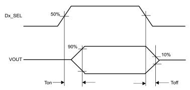
Figure 7-1. Select to Switch toon and toff
