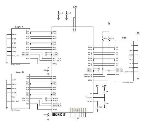
AUX\_SEL and Dx\_SEL configured for A to C
