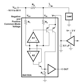
Figure 4. INA193A Example Shutdown Circuit
