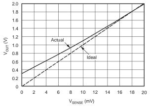
Figure 2. Example for Low V<sub>SENSE</sub> Cases 1 and 3 (INA195A, INA198A: Gain = 100)
