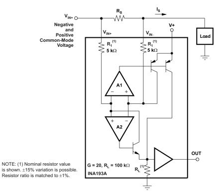
Figure 6. INA193A Simplified Circuit Diagram
