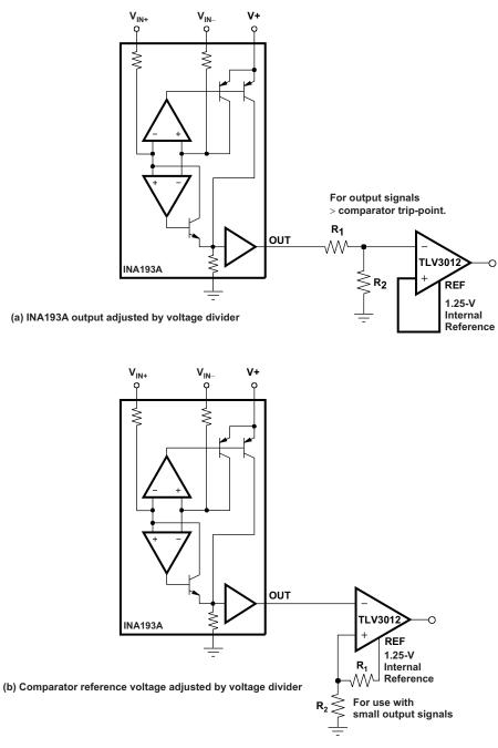
Figure 10. INA193A With Comparator
