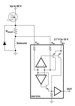
Figure 9. Inductive Current Monitor Including Flyback
