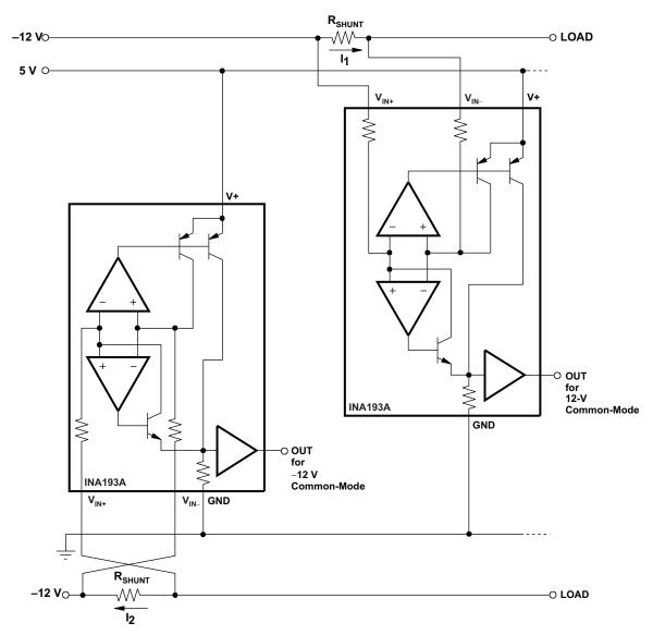
Figure 7. Monitor Bipolar Output Power-Supply Current
