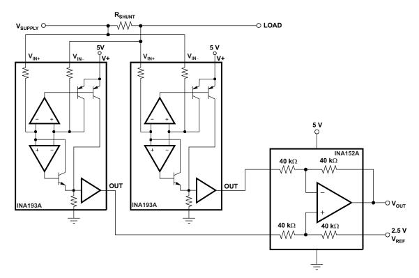
Figure 8. Bidirectional Current Monitoring
