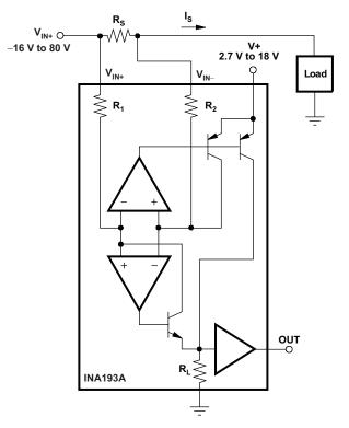
Figure 1. INA193A Basic Connection
