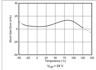
Figure 6-8. Shunt Input Gain Error vs. Temperature
