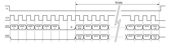
Figure 7-8. SPI Write Frame
