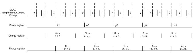
Figure 7-2. Power, Energy and Charge Calculation Scheme
