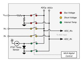
Figure 7-1. High-Voltage Input Multiplexer
