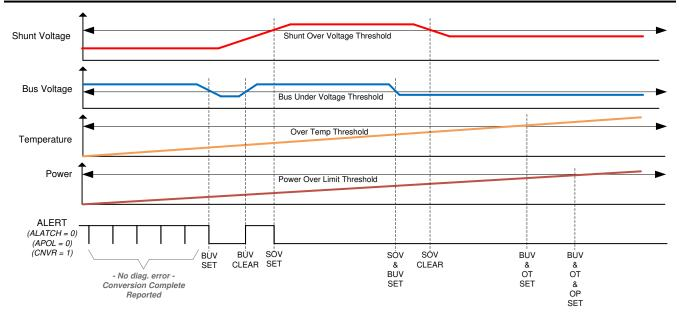
Figure 7-6. Multi-Alert Configuration
