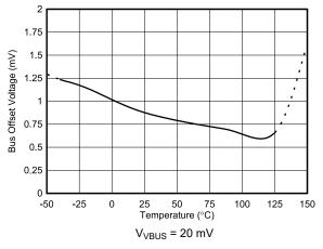
Figure 6-11. Bus Input Offset Voltage vs. Temperature
