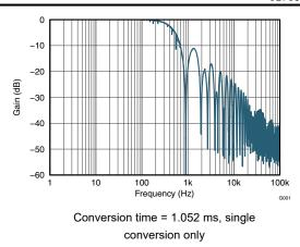
Figure 7-3. ADC Frequency Response
