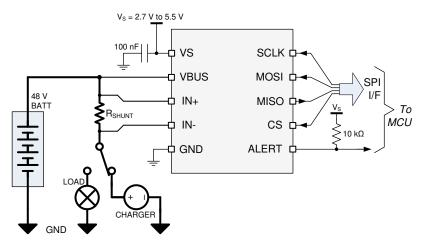
Figure 8-2. INA229 High-Side Sensing Application Diagram
