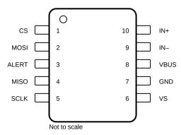
Figure 5-1. DGS Package 10-Pin VSSOP Top View
