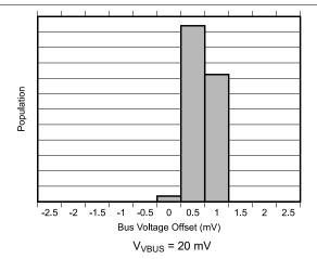
Figure 6-10. Bus Input Offset Voltage Production Distribution
