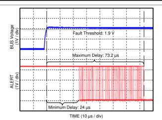
Figure 8-4. Alert Response Time (Sampled Values Slightly Above Threshold)
