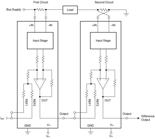
NOTE: The voltage applied to the reference inputs must not exceed 9 V.
