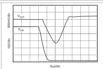
Figure 6-25. 50-V Common-Mode Step Response
