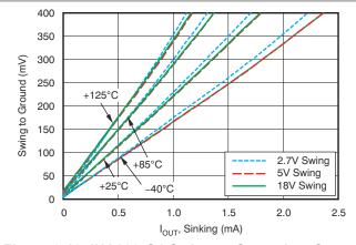
Figure 6-18. INA283-Q1 Swing to Ground vs Output Current
