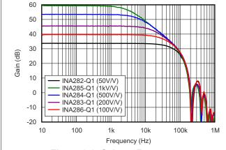
Figure 6-1. Gain vs Frequency
