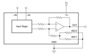
Figure 7-2. Ground Referenced Output
