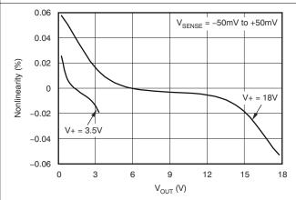
Figure 6-6. INA282-Q1 Typical Nonlinearity vs Output Voltage
