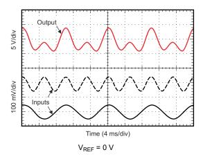
Figure 8-3. Current Summing Application Output Response
