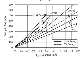
Figure 6-17. INA283-Q1 Swing to Rail vs Output Current
