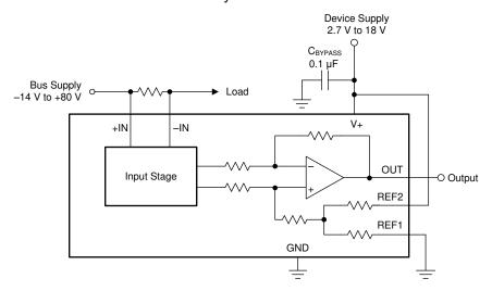
Figure 8-1. Basic Connections
