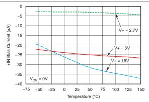
Figure 6-13. +IN BIAS Current vs Temperature
