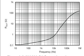
Figure 6-5. INA286-Q1 Output Impedance vs Frequency
