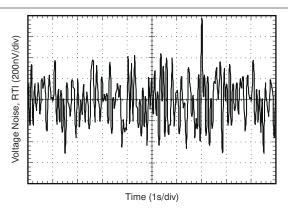
Figure 6-14. INA282-Q1 0.1-Hz to 10-Hz Voltage Noise, RTI
