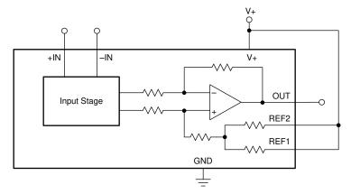
Figure 7-3. V+ Referenced Output
