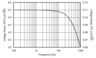
Figure 6-15. INA282-Q1 Voltage Noise vs Frequency
