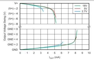
Figure 6-16. INA284-Q1 Output Voltage Swing vs Output Current
