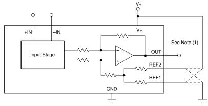
A. Reference divider accuracy is determined by measuring the output with the reference voltage applied to alternate reference resistors, and calculating a result such that the amplifier offset is cancelled in the final measurement.
