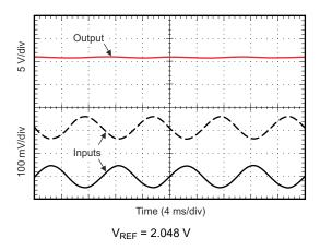
Figure 8-5. Current Differencing Application Output Response
