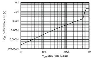
Figure 6-4. INA282-Q1 Common-Mode Slew Rate Induced Offset
