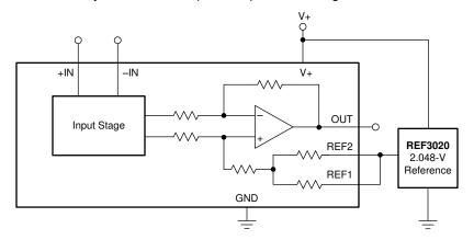
Figure 7-4. External Reference Output
