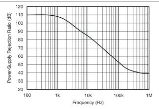
Figure 6-2. INA282-Q1 PSRR (RTI) vs Frequency
