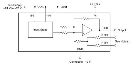
A. Connect the REF pins as desired; however, they cannot exceed 9 V greater than the GND pin voltage.
