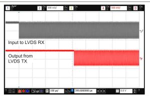
Figure 15. Distortion Correction Scheme Calibration Time  $(t_{CALIB})$
