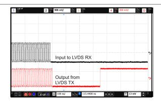
Figure 16. Transition From Valid Data to Idle ( $t_{IDLE\_OUT}$ )
