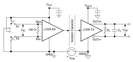
A.  $C_L = 5$  pF and includes instrumentation and fixture capacitance within  $\pm 20\%$ .
