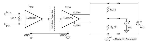
Figure 23. Driver Test Circuit
