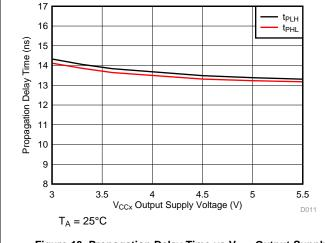
Figure 13. Propagation Delay Time vs V<sub>CCx</sub> Output Supply Voltage
