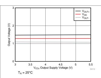
Figure 14. Output Voltage vs  $V_{\text{CCx}}$  Output Supply Voltage
