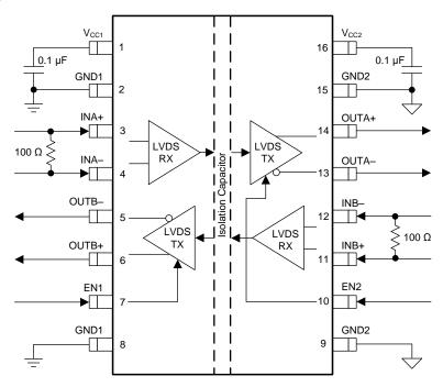
Figure 29. Typical ISO7821LLS Circuit Hook-Up
