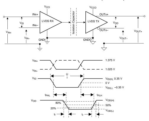
Figure 24. Voltage Definitions and Waveforms
