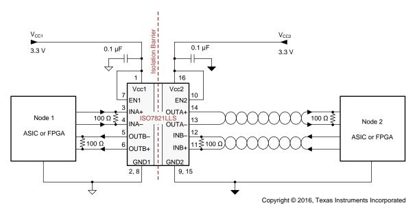
Figure 28. Isolated LVDS Interface Between Two Nodes (ASIC or FPGA)
