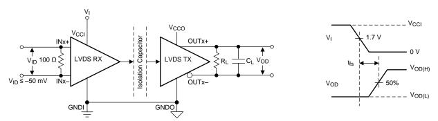
A.  $C_L = 5 \text{ pF}$  and includes instrumentation and fixture capacitance within  $\pm 20\%$ .
