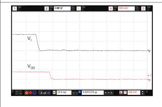
Figure 18. Disable Time ( $t_{PLZ}$ ,  $t_{PHZ}$ )
