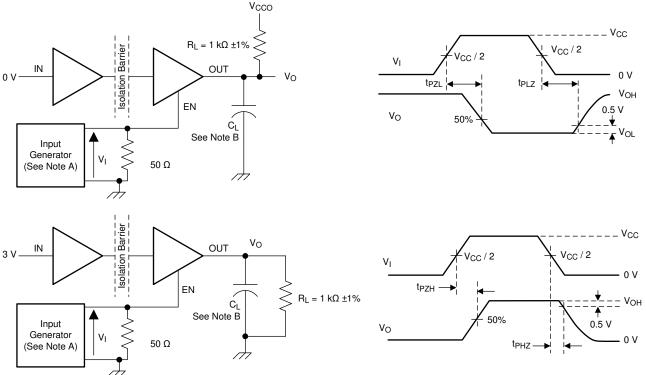
Figure 8-1. Switching Characteristics Test Circuit and Voltage Waveforms
