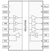
V<sub>CCI</sub>=Input supply, V<sub>CC2</sub>=Output supply GND1=Input ground, GND2=Output ground
