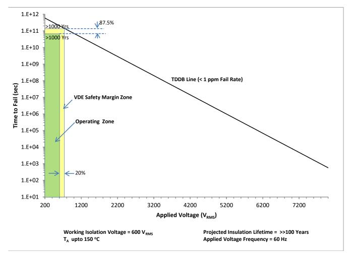
Figure 10-7. Insulation Lifetime Projection Data
