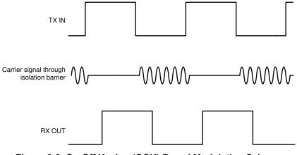
Figure 9-2. On-Off Keying (OOK) Based Modulation Scheme
