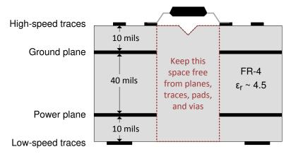
Figure 12-1. Layout Example Schematic
