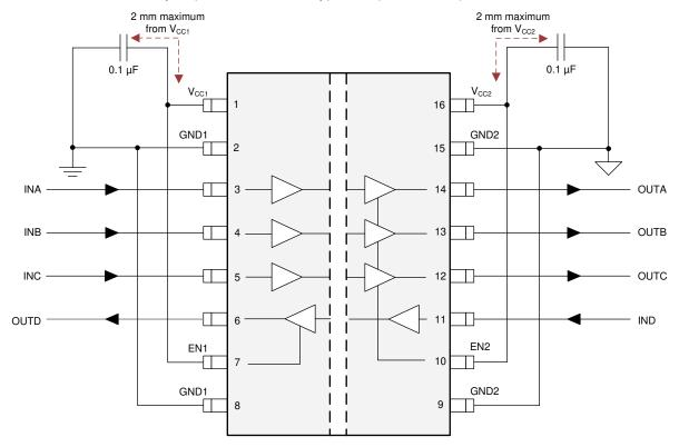
Figure 10-2. Typical ISOS141-SEP Circuit Hook-up
