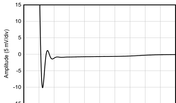
Figure 6-26. Small-Signal Step Response, G = 1
