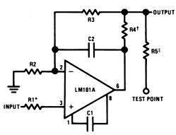
\*Protects input †Protects output ‡Protects output—not needed when R4 is used.
