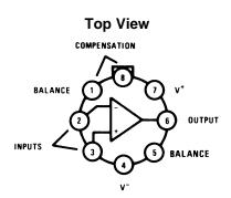
Figure 51. TO-99 Package See Package Number LMC0008C
