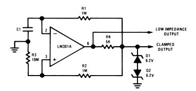
Figure 46. Low Frequency Square Wave Generator
