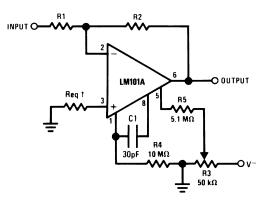
†May be zero or equal to parallel combination of R1 and R2 for minimum offset.
