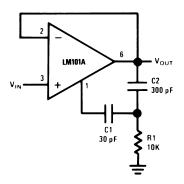
Power Bandwidth: 15 kHz Slew Rate: 1V/µs
