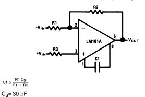
$C1 \geq \frac{R1 \ C_S}{R1 \ + \ R2}$ C<sub>S</sub>= 30 pF C2 = 10 C1
