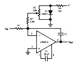
\*Adjust for zero integrator drift. Current drift typically 0.1 nA/°C over 0°C to +70°C temperature range.
