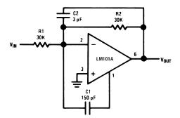
Power Bandwidth: 250 kHz Small Signal Bandwiidth: 3.5 MHz Slew Rate: 10V/µs
