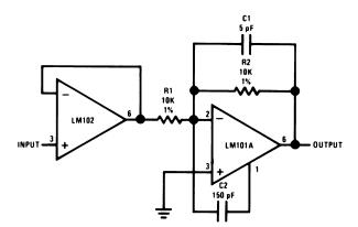
Figure 31. Fast Inverting Amplifier with High Input Impedance
