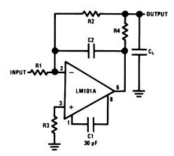
Figure 37. Isolating Large Capacitive Loads
