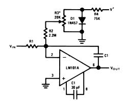
\*Adjust for zero integrator drift. Current drift typically 0.1 nA/°C over -55°C to +125°C temperature range.
