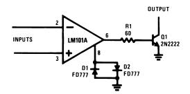
Figure 48. Voltage Comparator for Driving DTL or TTL Integrated Circuits
