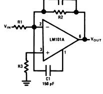
Figure 17. Single Pole Compensation
