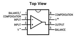
Figure 49. CDIP and PDIP Packages Package Number NAB0008A or P0008E
