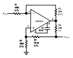
$I_{OUT} = \frac{\text{R3 V}_{\text{IN}}}{\text{R1 R5}}$ R3 = R4 + R5 R1 = R2
