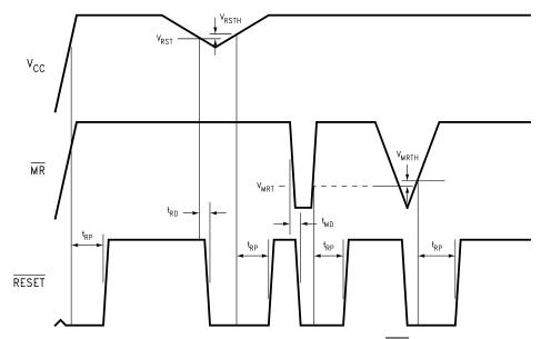
Figure 1. LM3704 Reset Time With MR
