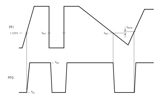
Figure 3. PFI Comparator Timing Diagram
