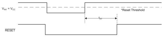
Standard reset threshold is 3.08 V. Custom reset voltages are available between 2.2 V and 5 V in 10-mV increments by contacting Texas Instruments.
