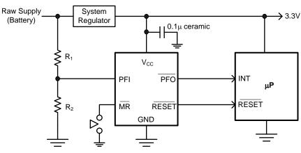
Power-Fail Reset Threshold,  $V_{PFT} = 1.225^{\circ} \left( \frac{R_1}{R_2} + 1 \right)$
