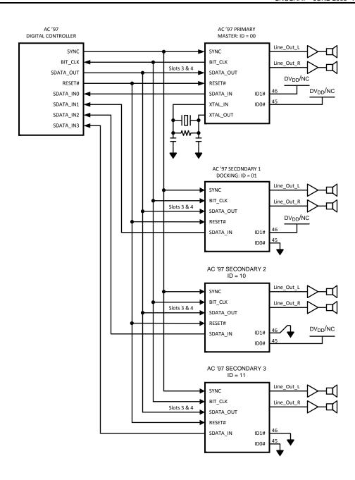
Figure 18. Multiple Codecs using Extended AC Link
