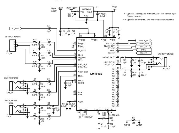
Figure 5. LM4546B Reference Design, Typical Application, Single Codec, 1 Vrms and 2 Vrms inputs, EMC output filters
