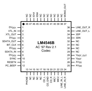
Figure 6. See Package Number PT0048A (Top View)
