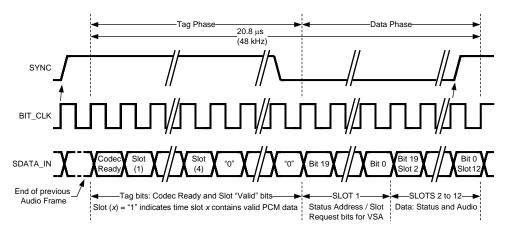
Figure 15. AC Link Input Frame
