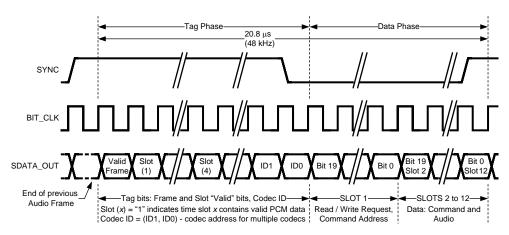
Figure 13. AC Link Output Frame
