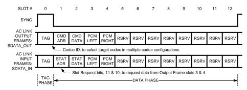
Figure 12. AC Link Bidirectional Audio Frame
