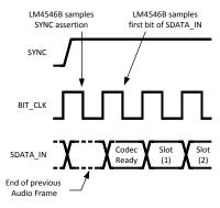
Figure 16. Start of AC Link Input Frame
