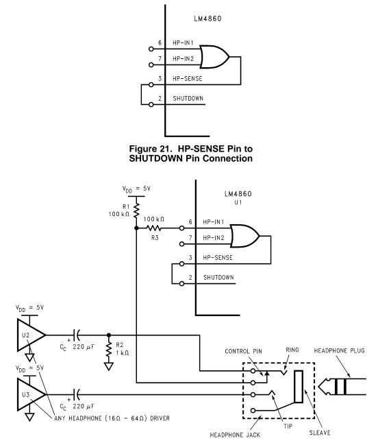
Figure 22. Typical Headphone Control Input Circuitry
