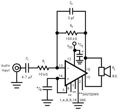
Figure 3. Stereo Amplifier with  $A_{VD} = 20$
