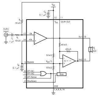
Figure 1. Typical Audio Amplifier Application Circuit
