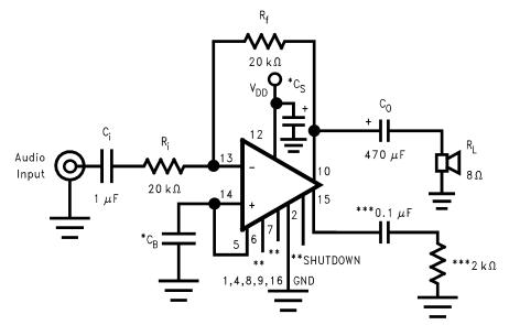
$C_S$  and  $C_B$  size depend on specific application requirements and constraints. Typical values of  $C_S$  and  $C_B$  are 0.1  $\mu$ F. \*\*Pin 2, 6, or 7 should be connected to  $V_{DD}$  to disable the amplifier or to GND to enable the amplifier. These pins should not be left floating.
